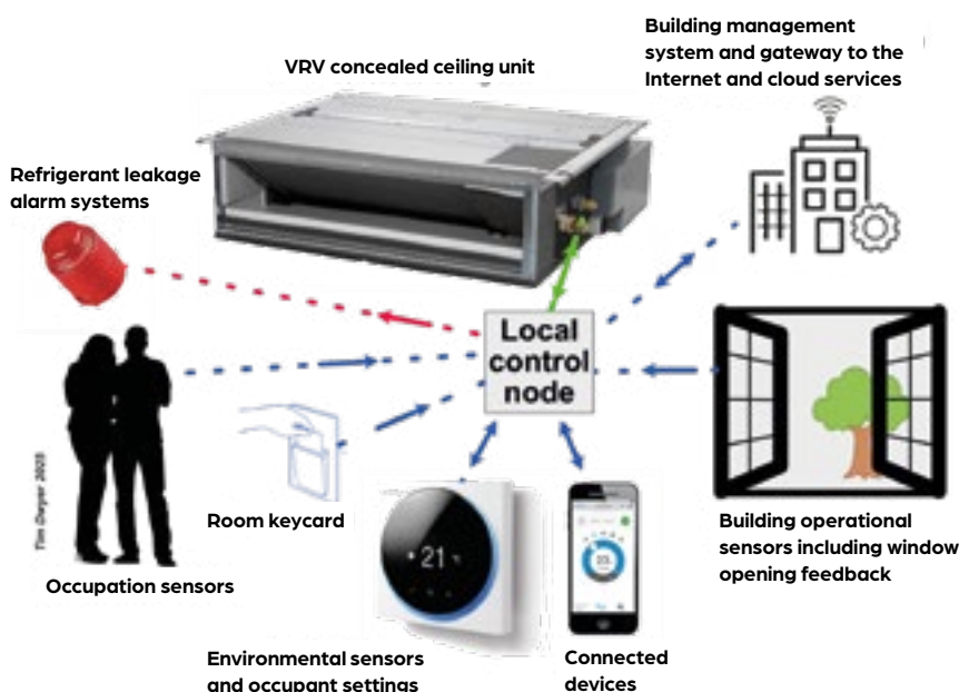
Figure 1: An example of a VRF room unit with integrated refrigerant leak sensor. Detection of a leak automatically isolates the connected refrigerant circuit and activates a local alarm. The environmental monitoring and control of the unit can be linked to a suitable selection of inputs and outputs – both local and cloud-based
