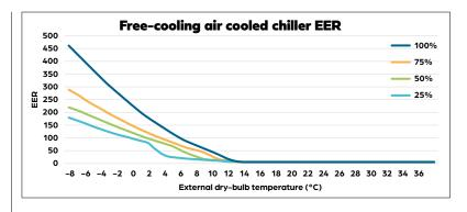
Figure 1: Example of true FC-ACC EER performance varying with temperature and part-loading
