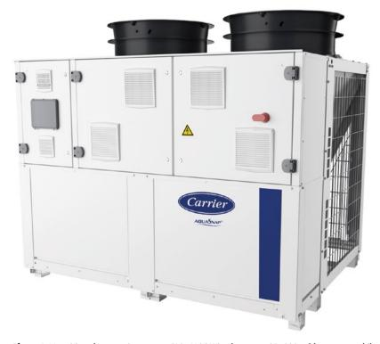
**Figure 1:** Monobloc air source heat pump (40–140 kW) using natural R–290 refrigerant, providing heating up to 75°C and operation down to –25°C outdoor temperature, with seasonal coefficient of performance (SCOP) up to 4.20 and energy efficiency up to 30% above Ecodesign requirements (Source: Carrier)
