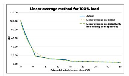
Figure 3: Actual and linear average prediction of EER varying with external temperatures when at 100% load
