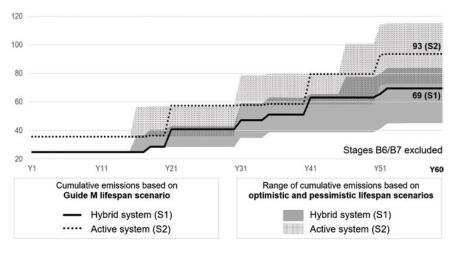
Figure 4: Life–cycle embodied carbon emissions over 60 years (kg  $CO_2e \cdot m^{-2}GIA$ )
