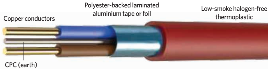
Figure 3: A simplified sketch of an example fire-resistant polymeric cable. There are many variants of such cables that are designed to meet specific fire-resistance requirements
