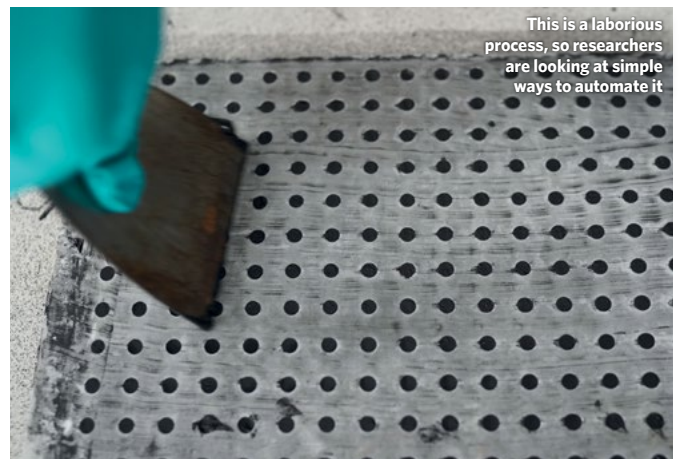
Applying the Alginate/graphite paste into a silicon mould to create a consistent shape and size of bead.
