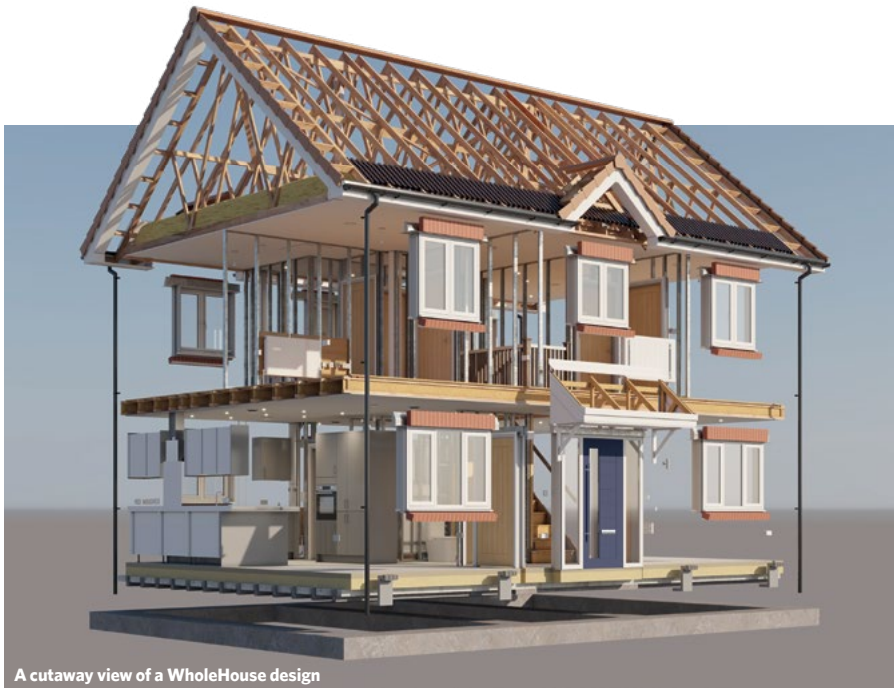
A cutaway view of a WholeHouse design
