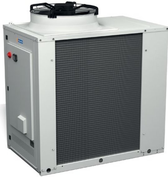
Figure 1: Monobloc R32, 50kW, air source heat pump with inverter-controlled compressor with COP up to 4.11@water 35°C, air 7°C, SCOP 4.16@35°C, 3.08@55°C. 1.920m wide, 1.110m deep, 1.920m high, 535kg (Source: Hamworthy)
