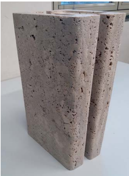
Pavilion building façade visual mock-up and CNC travertine fin prior to surface filling
