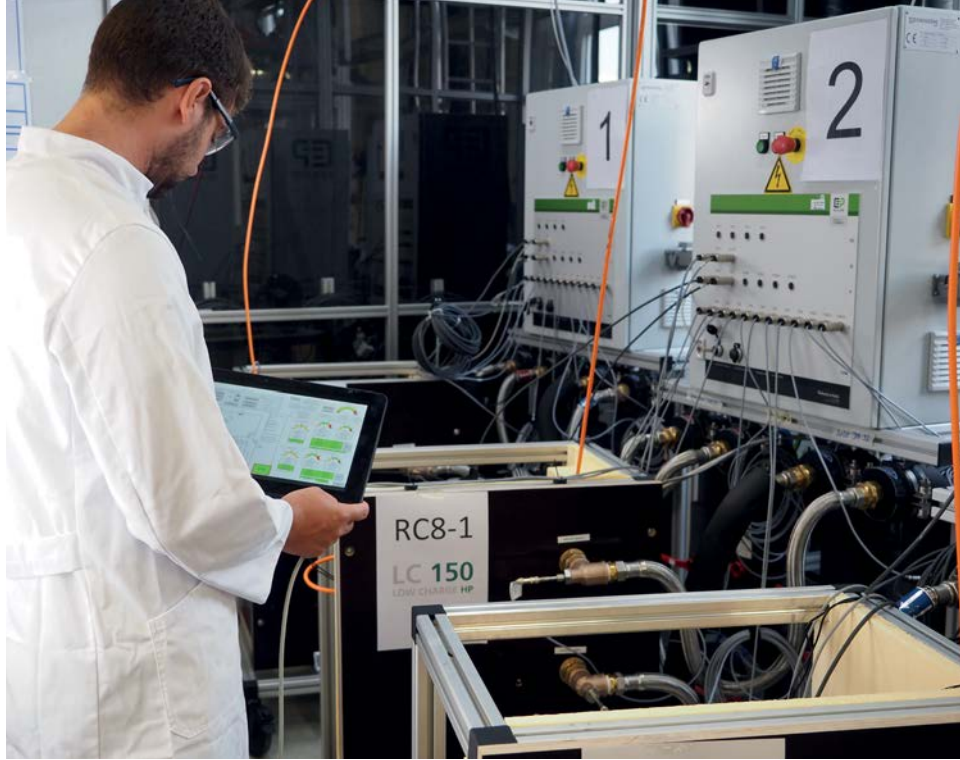
Heat pump test rigs running 24 hours a day
