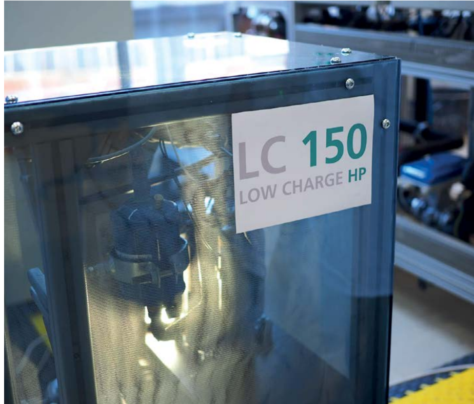
The LC150 heat pump, developed at Fraunhofer ISE, is based on the climate-friendly refrigerant propane
