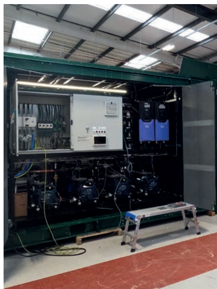
A CO 2 heat pump in the factory destined for a school
