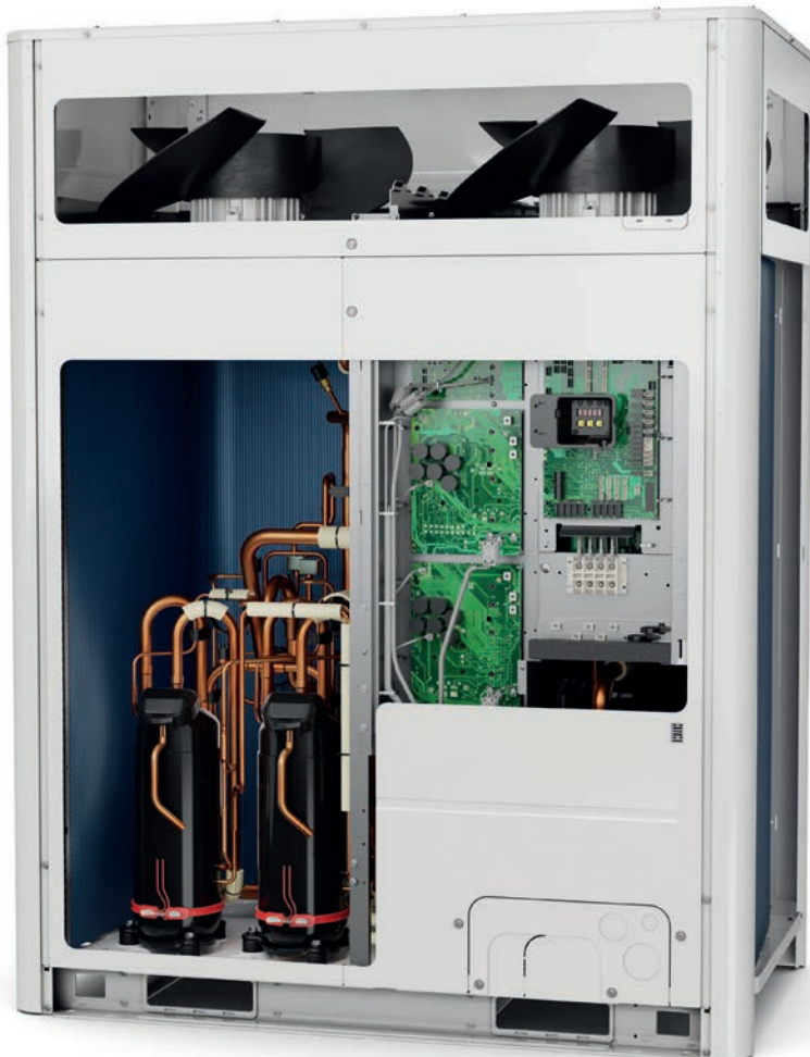
Figure 1: Example of recently developed external unit for variable refrigerant flow (VRF) system, operating with a R-32 twin-rotary compressor with liquid injection, split heat exchanger, sub-cooling plate heat exchanger, a high-performance fan motor, and novel control features, all contributing to providing a SEER up to 8.9 and SCOP up to 4.67
