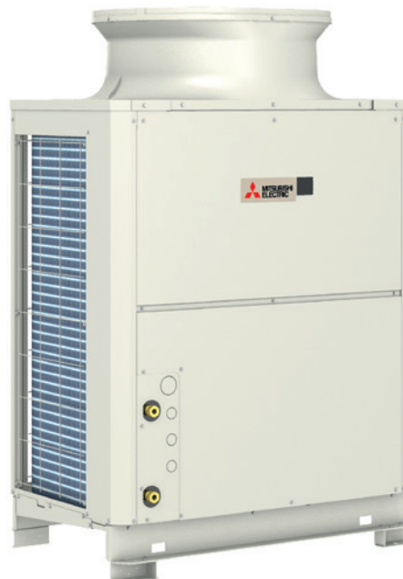
Figure 1: Example of commercially available air source heat pump designed for commercial domestic hot water application, where gas boilers, combined heat and power systems (CHP) or electric water heating have been traditionally utilised. At outdoor 7°CDB/6°CWB, inlet water temperature 9°C, the unit produces 40kW of water at 65°C with a COP of 3.65 (1,220mm x 760mm x 1,837mm high)
