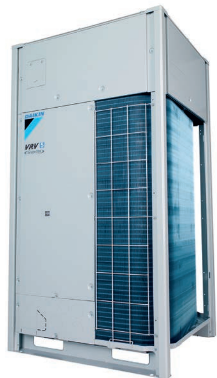
Figure 3: An example of an inverter-controlled external unit supplying VRV (VRV) internal units with integrated refrigerant safety measures and heat recovery, employing R32. This range delivers up to 90kW heating capacity (@indoor 20°C DB, outdoor 7°C DB, 6°C WB) and 80kW cooling (@indoor 27°C DB/19°C WB, outdoor 35°C DB) with standardised SEER 7.1, SCOP 4.1 (Source: Daikin 21 )
